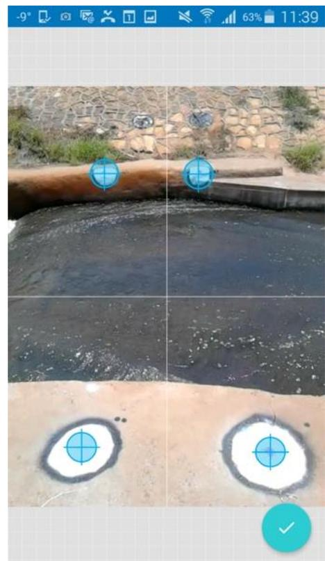
The water level is picked by moving the blue line to the actual water level. Pinching will zoom into the image, making it easier to click the water level accurately. As the user slides the water level up and down, in the lower part of the image the water level in metric units is shown.
