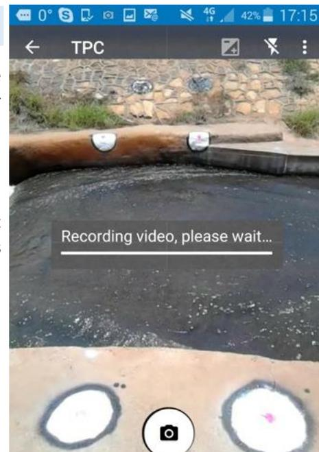
After the video is recorded, the app shows the screen which asks the user to select the location of the GCPs. For each GCP the user needs to move the blue hair cross exactly over the site GCP. For now, the 'adjust GCP size' feature can be ignored (later version will use this feature for automatic GCP detection).
