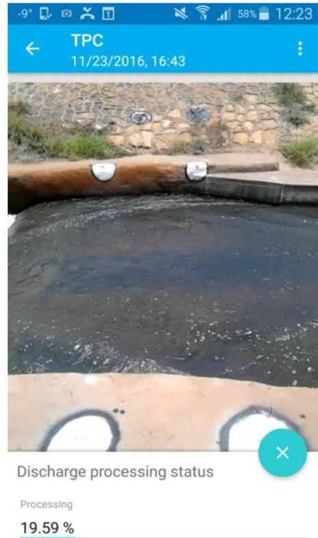
After the processing is done, the velocity vectors are rendered, as well as the calculated discharge, velocity and water height. By clicking the cloud button, the measurement is sent to the web-platform.
