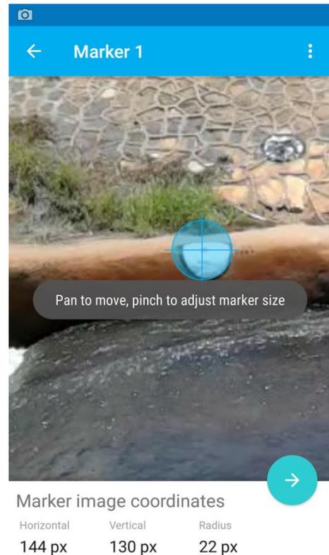
After positioning the four GCPs, a last control view appears and by pressing the checkmark the app will calibrate the view, i.e. it will determine the device position and orientation relative to the site. This will take only an instant and then the menu will move on to the level picking step.
