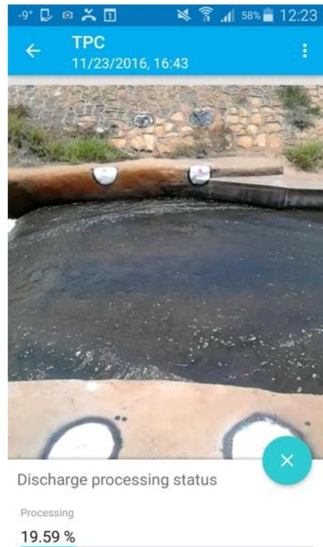
After the processing is done, the velocity vectors are rendered, as well as the calculated discharge, velocity and water height. By clicking the cloud button, the measurement is sent to the web-platform.
