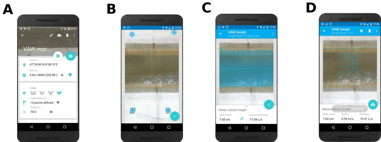
Figure 3. Four main steps required to apply the DischargeApp . (A) Site selection and configuration. (B) After the video recording, manual definition of the location of the ground control points. (C) User guided determination of the actual water level. (D) Results obtained after measuring the water level, the surface velocity field and after processing the data to compute the discharge.
